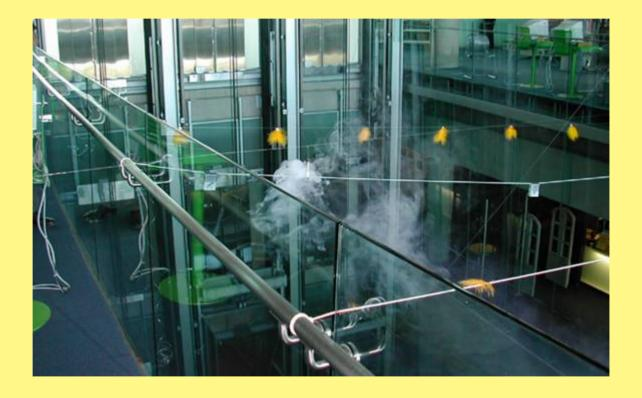
A smoke stick was attached to a line and moved across the atrium opening at the 5<sup>th</sup> level.
