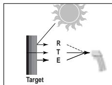
Infrared thermometers measure the surface temperature of an object. The unit's optics sense emitted (E), reflected (R), and transmitted (T) energy, which is collected and focused onto a detector. The unit's electronics translate the information into a temperature reading which is displayed on the unit. In units with a laser, the laser is used for aiming purposes only.
